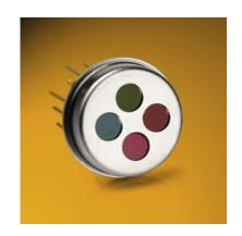
Multi-channel detectors are most commonly found in gas sensing applications as when combined with narrow bandpass IR filters targeted at specific gas lines; incredibly compact gas sensors can be made based on NDIR detection methods.
